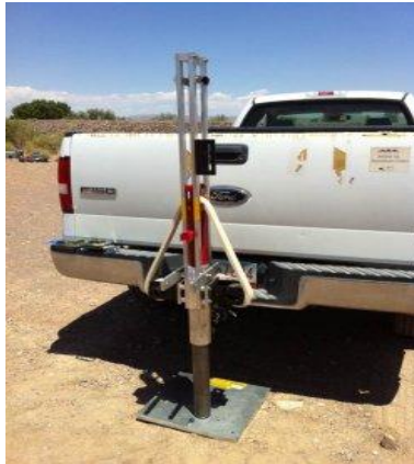
Fig.18: Testing with the dropping weight
