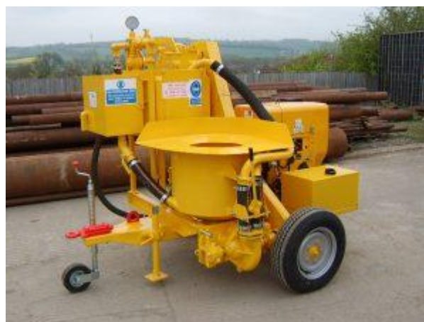
Figure 10: Grout mixer with integrated grout pump
