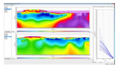
The picture is showing the resistivity and IP models for a 2D profile, and IP decay curves.
