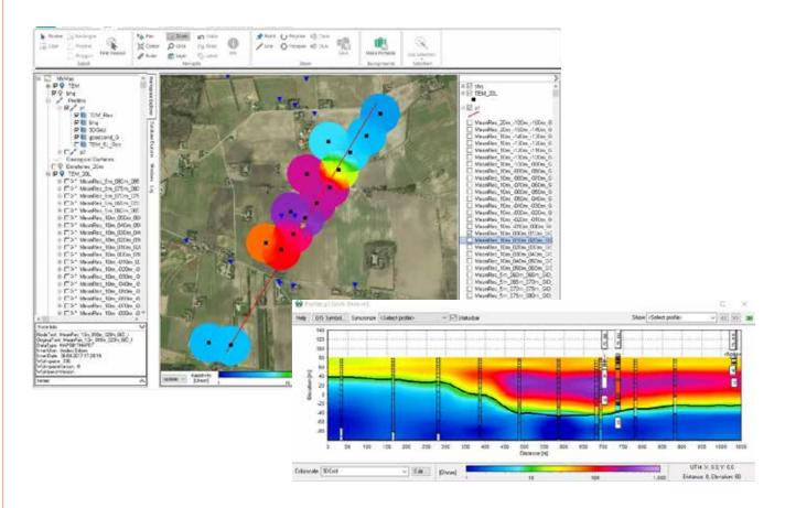
Multiple soundings measured in Aarhus, Denmark using an ABEM WalkTEM. Data was collected for geological mapping of a buried valley where groundwater is located.
