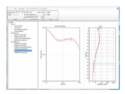
Resistivity sounding measured in Arusha, Tanzania using an ABEM Terrameter SAS1000. Data was collected in a groundwater survey as a pre-investigation for a well drilling.
